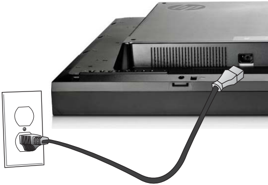
Figure 3-23 HP LD4720tm—Connecting the power cord
