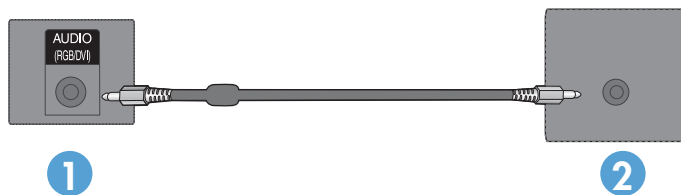
Figure 3-27 Connecting the audio cable
