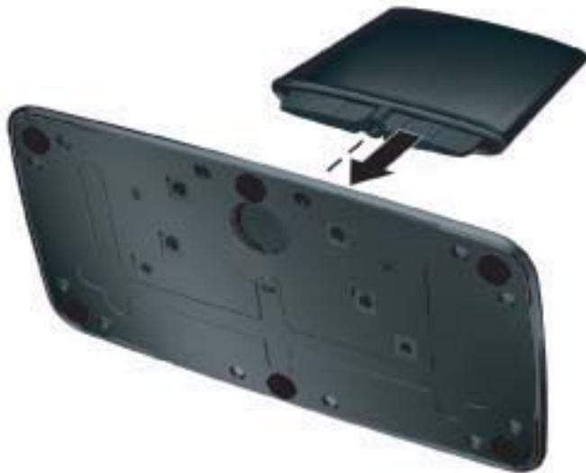
3. Slide the hinge bracket on the monitor into the opening on top of the pedestal. The panel will click into place when fully inserted.
