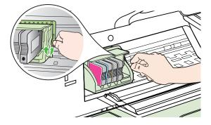
4. Remove the printhead by lifting it up and then pulling it out of the printer.
