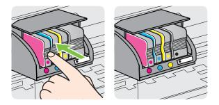
Make sure that you insert the ink cartridge into the slot that has the same colored letter as the color you are installing.
