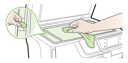
▲ CAUTION: Use only glass cleaner to clean the scanner glass. Avoid cleaners that contain abrasives, acetone, benzene, and carbon tetrachloride, all of which can damage the scanner glass. Avoid isopropyl alcohol because it can leave streaks on the glass.
