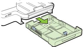
2. Insert the media print-side down in the center of the tray. Make sure the stack of media aligns with the line on the width guide, and is not higher than the paper stack line on the guide.
