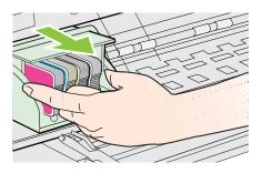
5. Make sure the latch handle is raised, and then reinsert the printhead.
