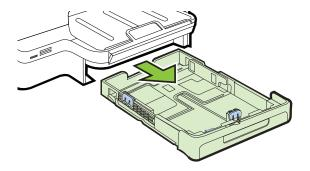
2. Insert the envelopes print-side down and load according to the graphic. Make sure the stack of envelopes does not exceed the line marking in the tray.
