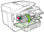
3. Lift the latch handle on the print carriage.
