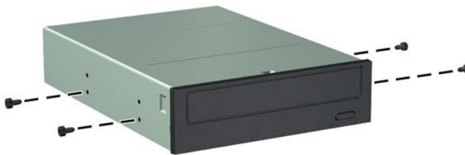
Figure 5-15 Installing Guide Screws in the Optical Drive
