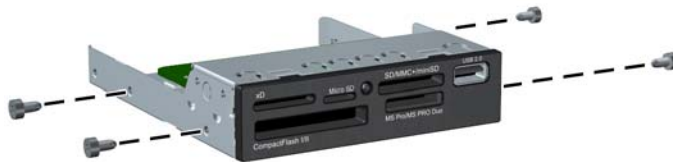
Figure 5-19 Installing Guide Screws (Media Card Reader Shown)
