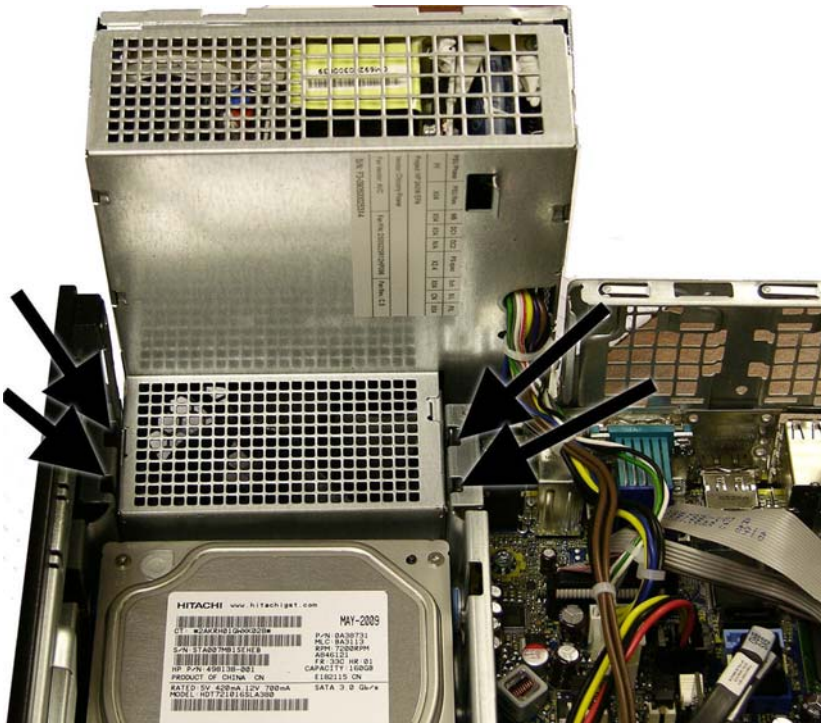
Figure 5-37 Removing the power supply
