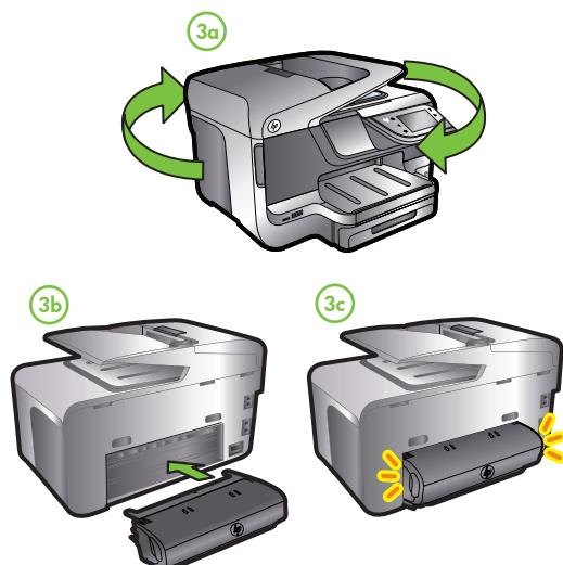
(EN) Install the HP automatic two-sided printing accessory (duplexer).
