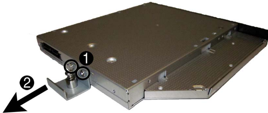
Figure 7-12 Removing the optical drive bracket
