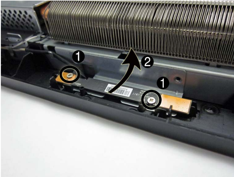
Figure 7-5 Removing the webcam module
