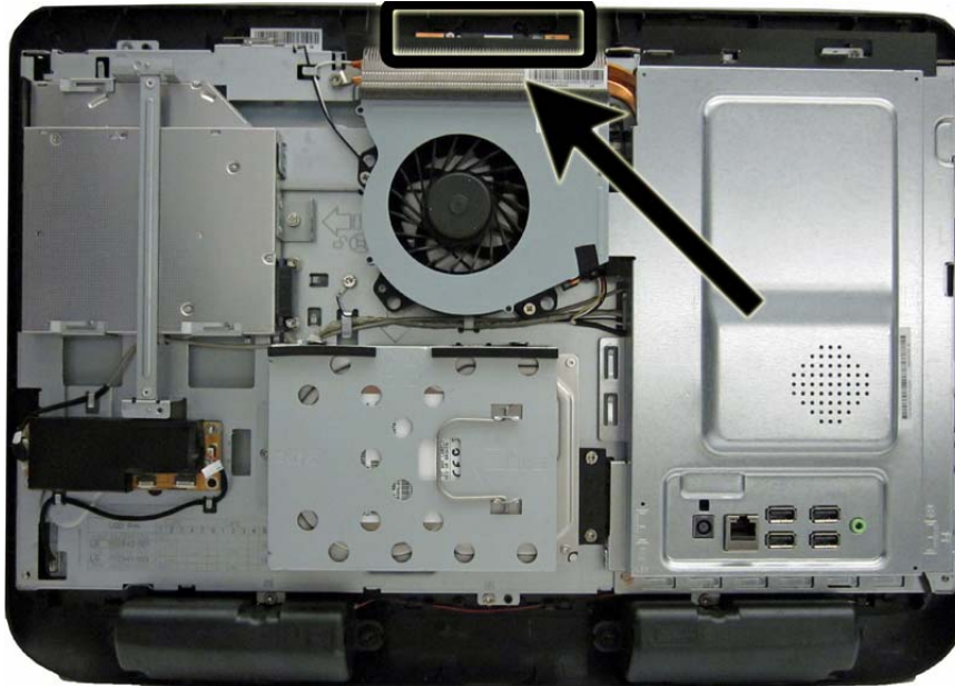
Figure 7-4 Webcam module location
