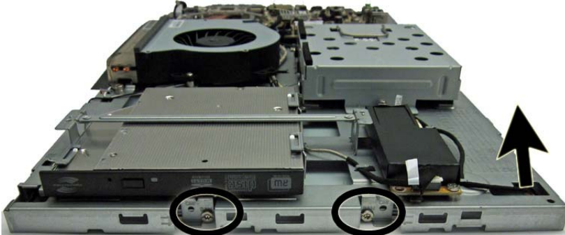
Figure 7-40 Removing the display panel screws and converter cable
