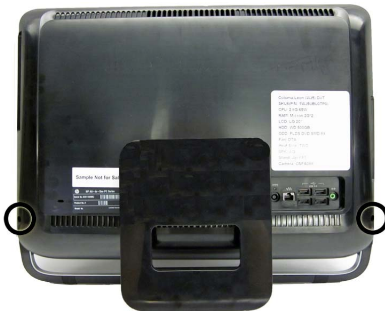
Figure 7-1 Removing the rear cover screws
