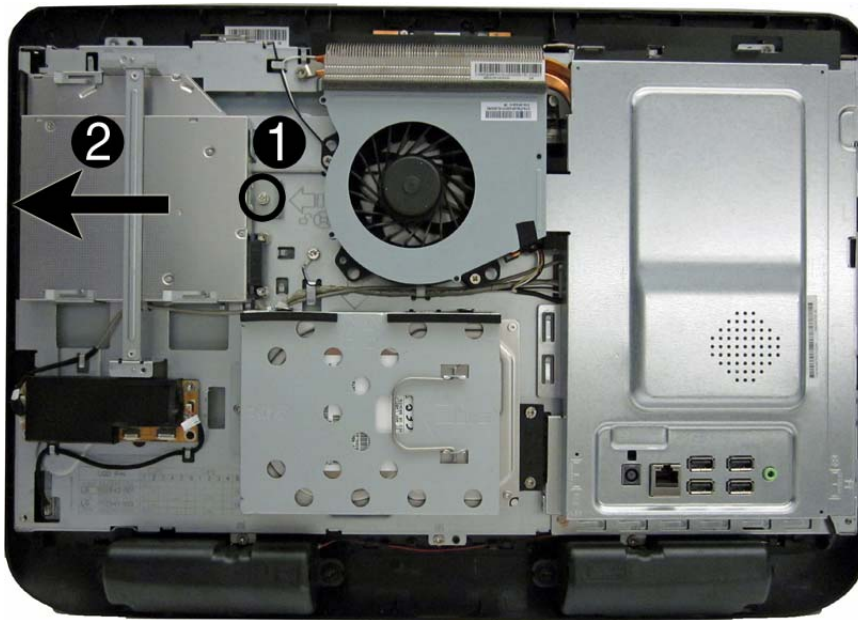
Figure 7-11 Removing the optical drive
