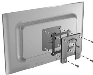
When assembling the monitor panel to an Integrated Work Center Stand, install the HP accessory plate to the rear of the monitor panel and then, attach the Quick Release. The accessory plate will fill the gap between the monitor and the quick release bracket to fit flush onto the rear of the monitor. The accessory plate is recommended for HP monitor models LA2006x, LA2206x, LA2206xc, and LA2306x that are installed on the integrated work center stand.
