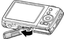
3. Insert the battery into the compartment with correct orientation as illustrated. Be sure to push the battery into position until the battery is locked into place.
