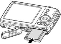
4. Close and secure the battery/memory card compartment by sliding the locking button towards the edge of the camera (as illustrated).
