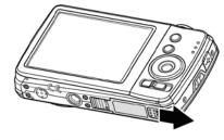
2. Open the battery/memory card compartment at the bottom of the camera by sliding the locking button towards the center as illustrated.
