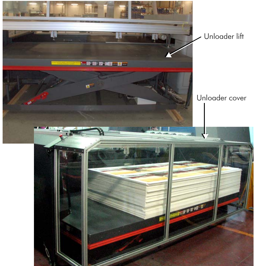
Figure 2-27 Unloader Lift with Open/Closed Cover
