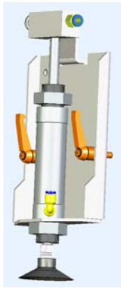
Figure 2-24 Loading/Unloading Suction Cup
