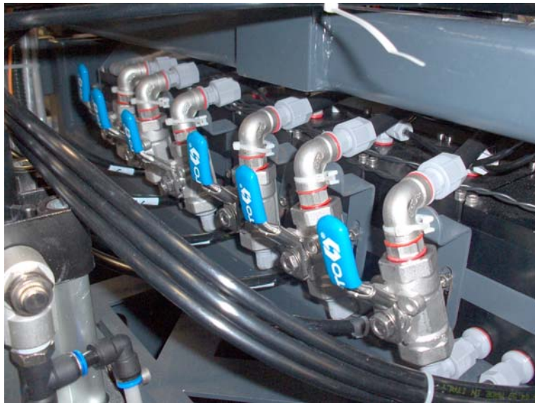
Figure 2-12 Secondary Ink Tanks with Taps
