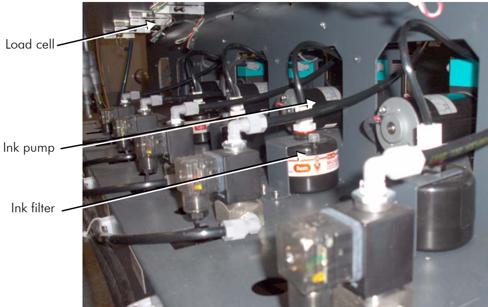
Figure 2-14 Ink System Components
