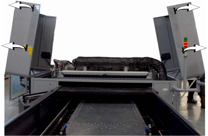
Figure 8-1 Raising the Bridge Upper Hoods
