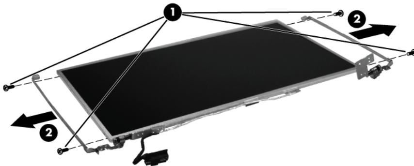
Reverse this procedure to install the display hinges.
