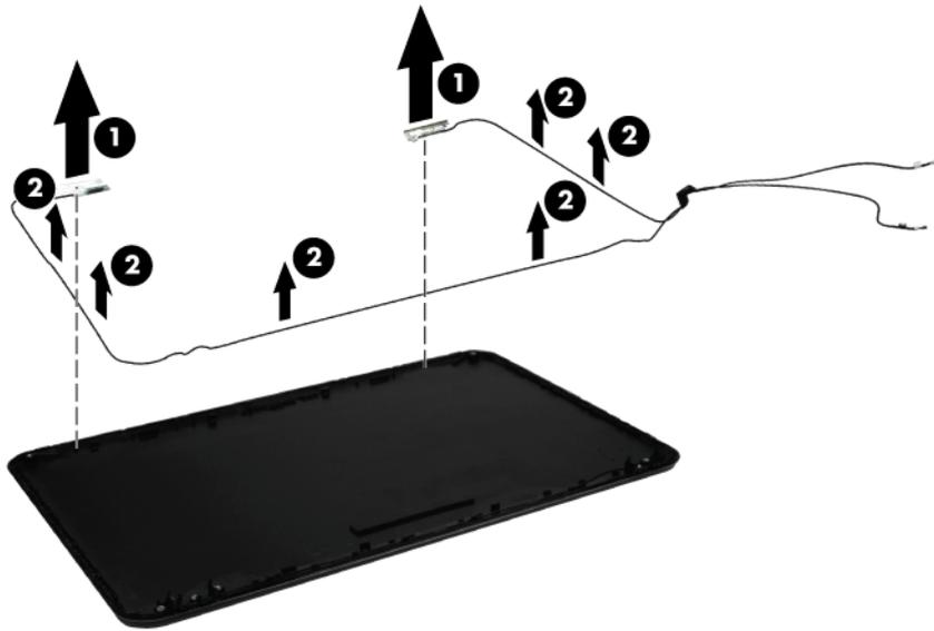
Reverse this procedure to install the display wireless antenna transceivers.
