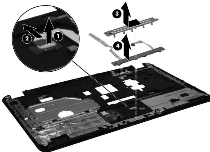
Reverse the above procedure to reassemble and install the TouchPad button board.
