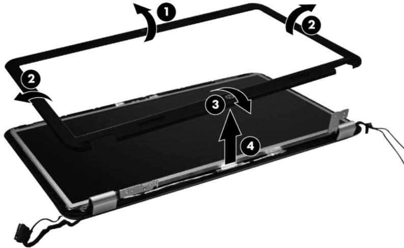
Reverse this procedure to install the display bezel.
