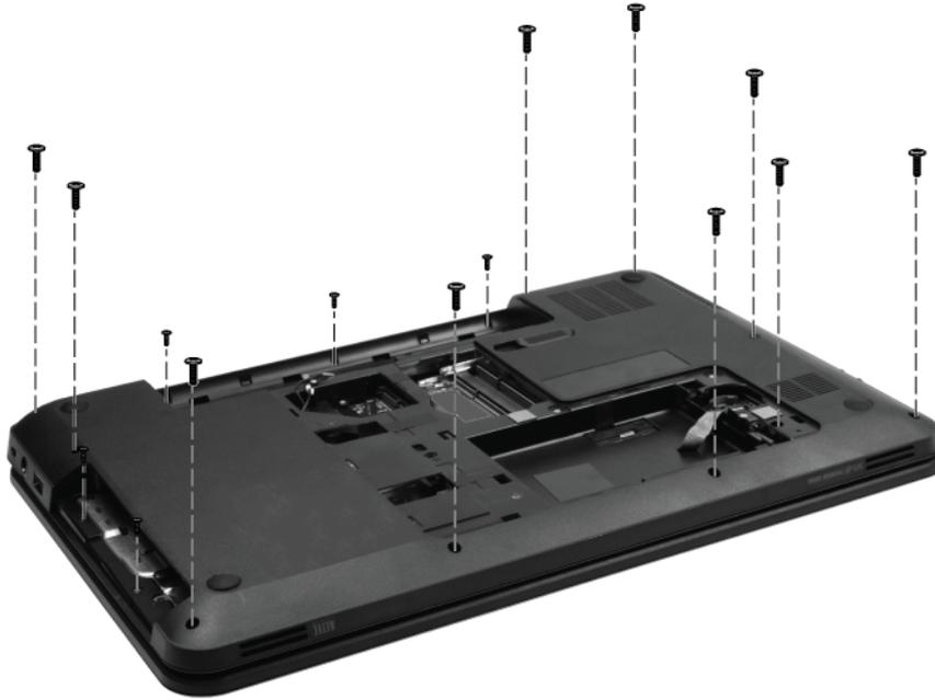
6. Lift the rear edge of the top cover **(1)** until the top cover disengages from the base enclosure. Remove the top cover **(2)**.
