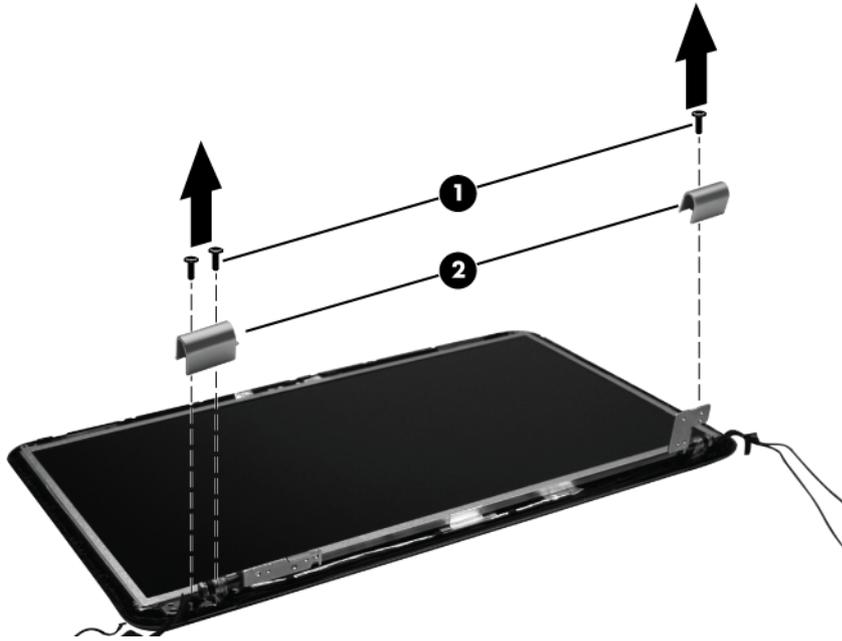
Reverse this procedure to install the display hinge covers.
