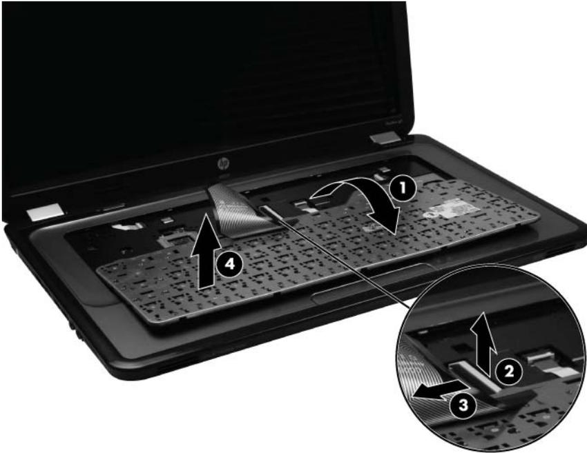
Reverse this procedure to install the keyboard.
