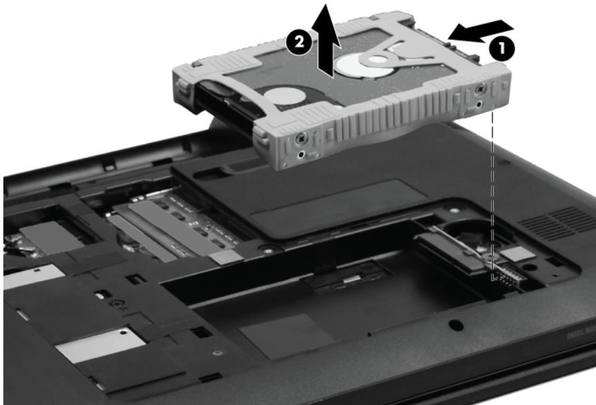
3. To replace the hard drive bracket, remove the four Phillips 3.0x3.0 screws **(1)** that secure the hard drive bracket to the hard drive.
