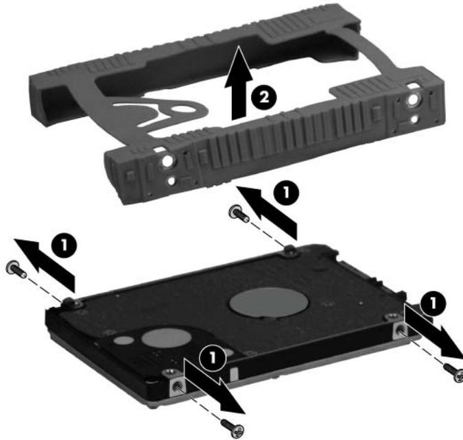
5. To replace the hard drive adapter, remove the Phillips pan head 2.0 x 2.0 screw **(1)**, and then disconnect the adapter from the system board at the outside edge **(2)**.
