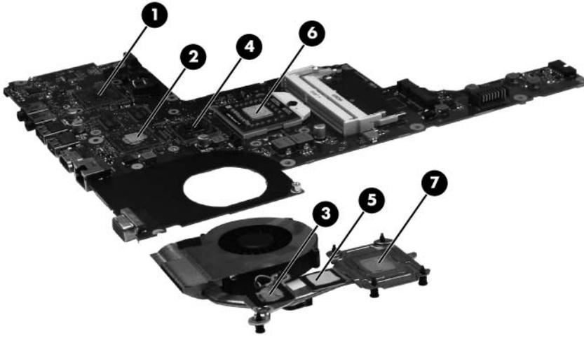
After applying fresh thermal paste to the components, reverse the above procedure to install the fan/heat sink assembly.
