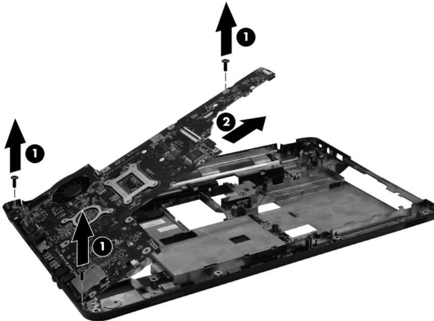
When replacing the system board, be sure that the following components are removed from the defective system board and installed on the replacement system board:
