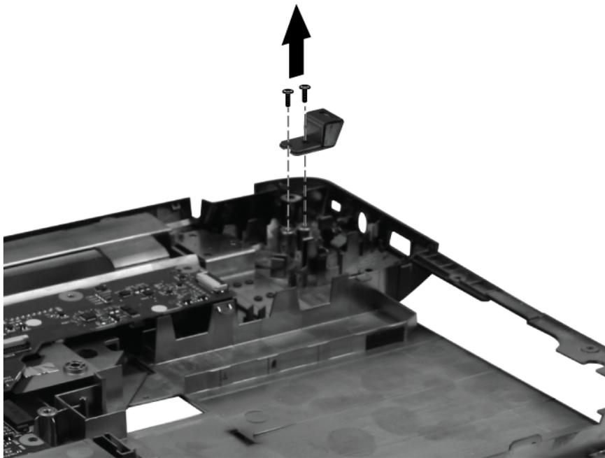
Reverse this procedure to install the security cable lock.
