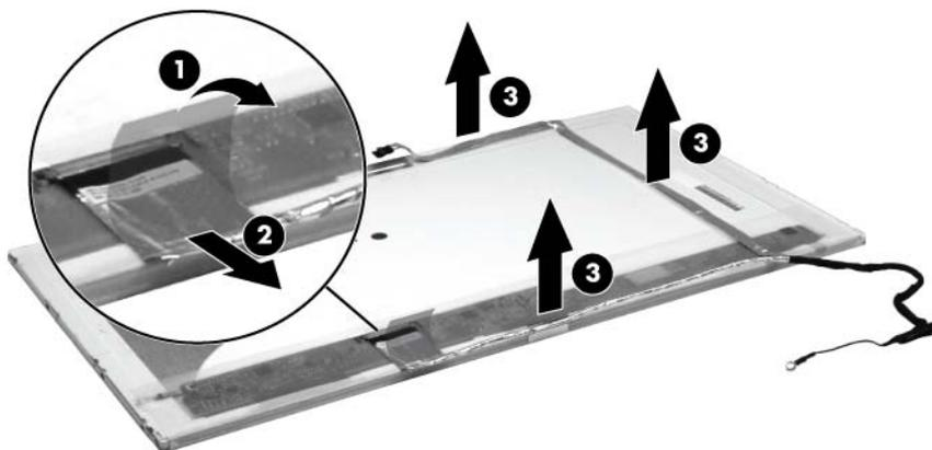
Reverse this procedure to install the display panel.
