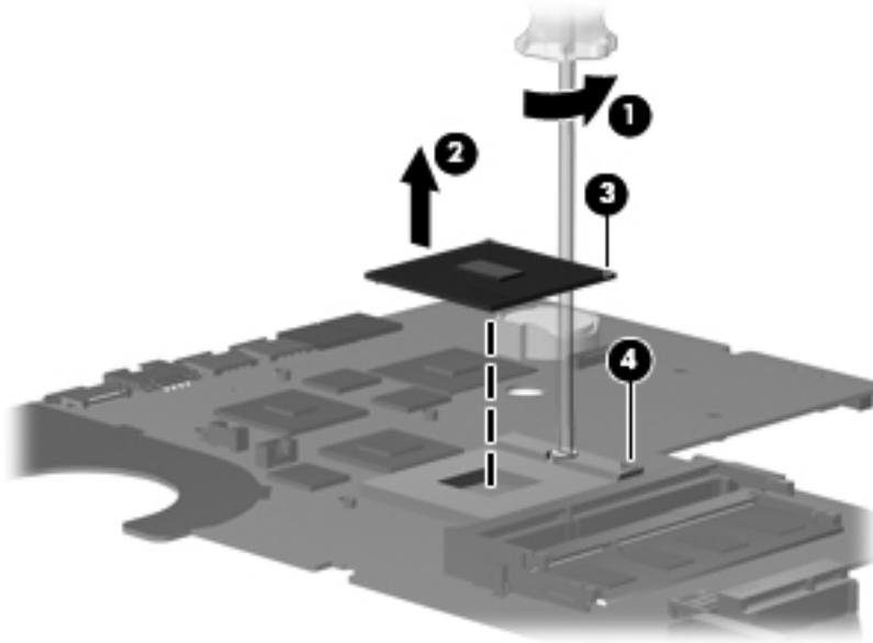
Reverse this procedure to install the processor.
