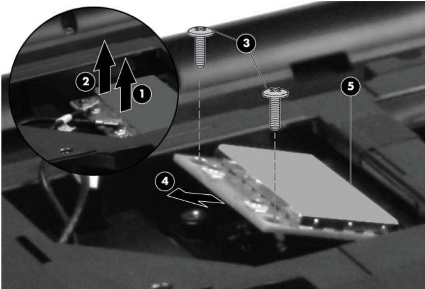
Reverse this procedure to install a WLAN module.
