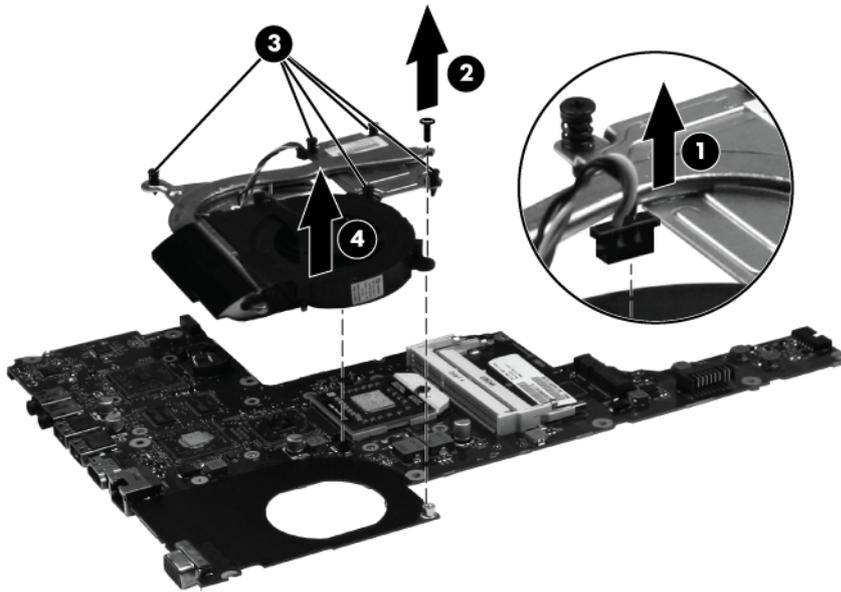
Each time the fan/heat sink assembly is removed, the thermal material must be thoroughly cleaned from the system board at locations (1) and (2), from the fan/heat sink assembly at locations (3) and (5), and from the processor (4). Thermal pads and thermal paste must be installed on all surfaces before the fan/heat sink assembly is reinstalled.
