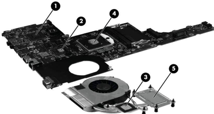
Each time the fan/heat sink assembly is removed, the thermal material must be thoroughly cleaned from the system board at locations (1), (2), and (4), from the fan/heat sink assembly at locations (3), (5), and (7), and from the processor (6). Thermal pads and thermal paste must be installed on all surfaces before the fan/heat sink assembly is reinstalled.
