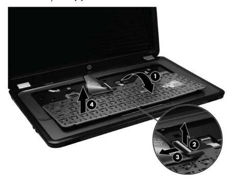
Reverse this procedure to install the keyboard.
