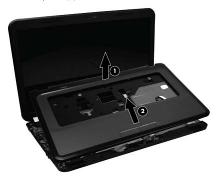
NOTE: The TouchPad is glued to the top cover and is included with the top cover spare part.
