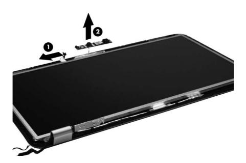
Reverse this procedure to install the webcam module.
