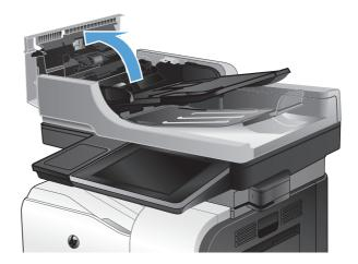
3. Remove any visible lint or dust from each of the feed rollers and the separation pad using compressed air or a clean lint-free cloth moistened with warm water.
