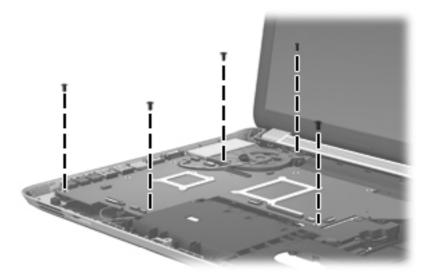
Reverse this procedure to install the SD Card reader board and cable.
