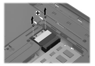
3. Remove the WLAN module by pulling the module away from the slot at an angle.
