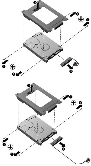
NOTE: The hard drive connector cable used on the secondary hard drive has a longer cable.
