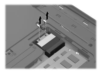
2. Remove the two Phillips PM2.0×4.0 screws that secure the WLAN module to the system board. (The WLAN module tilts up.)
