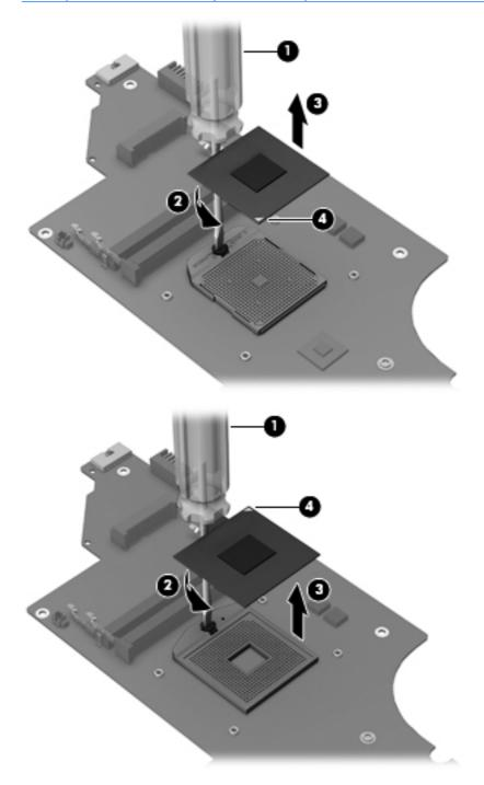
Reverse this procedure to install the processor.
