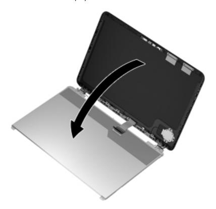
c. Release the adhesive strip (1) that secures the display panel cable to the display panel, and then disconnect the display panel cable (2) from the display panel.
