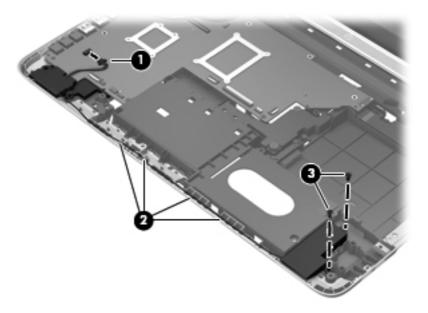
Rotate the front left speaker (1) clockwise to release it from under the system board.
