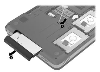
5. Push on the hard drive bracket (1) to release the optical drive.
