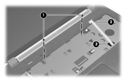
Lift the rear edge of the top cover (1) until the left and right sides disengage from the base enclosure.
