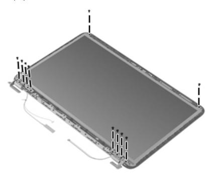
**b.** Lift the top edge of the display panel, and then swing it up and forward until it rests upside down in front of the display enclosure.
