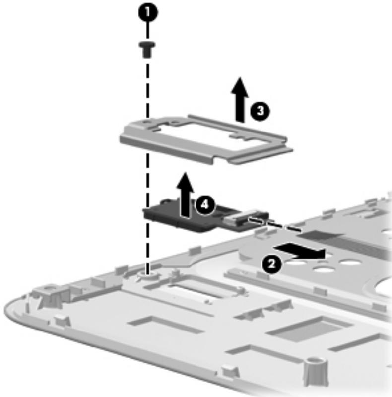
Reverse the above procedure to install the fingerprint reader board.
