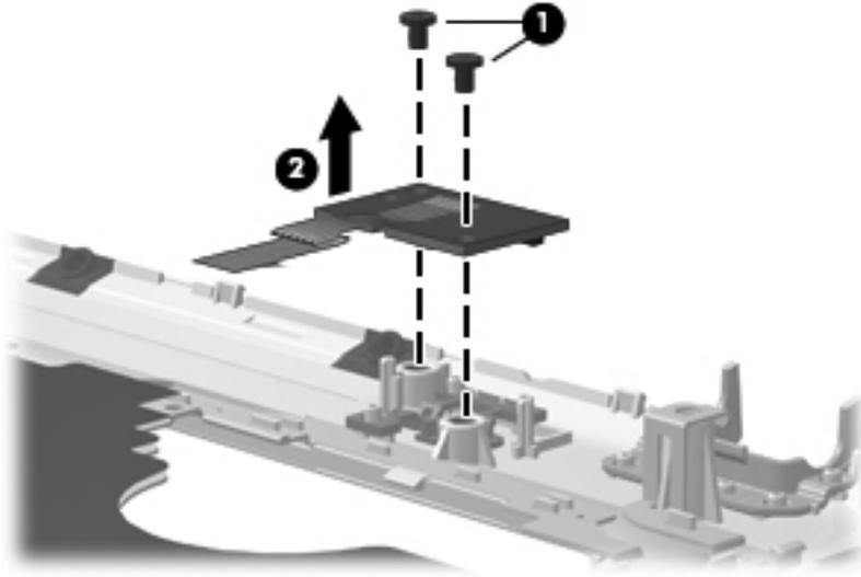
Reverse the above procedure to install the power button board.
