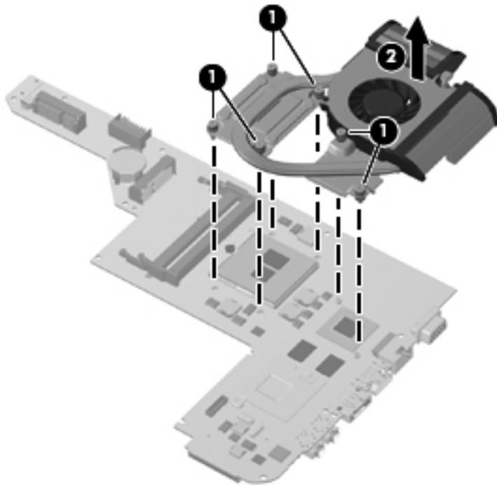
The thermal material must be thoroughly cleaned from the surfaces of the fan/heat sink assembly (1), (3) and the processor (2) and graphics processor (3) on the system board each time the fan/heat sink assembly is removed. Thermal pads and thermal paste must be installed on all surfaces before the fan/heat sink assembly is reinstalled.
