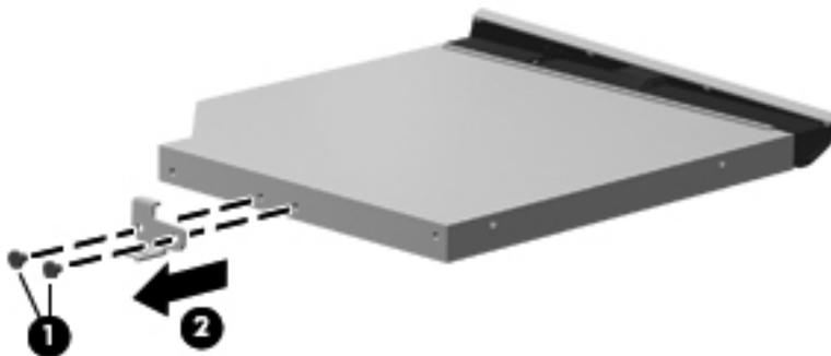
Reverse the above procedure to reassemble and install the optical drive.
