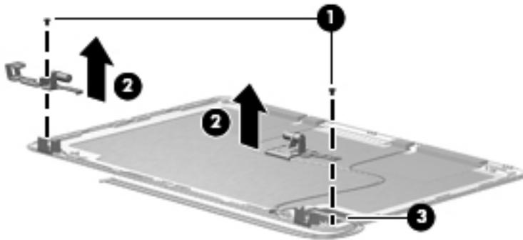
17. If it is necessary to replace the wireless antennas and cables, remove the adhesive strip **(1)** that secures each antenna to the display back cover.
