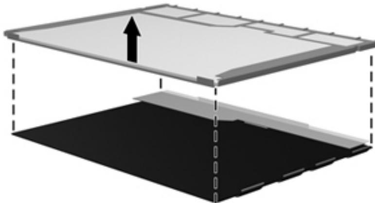
24. Recycle the LCD panel and backlight.
