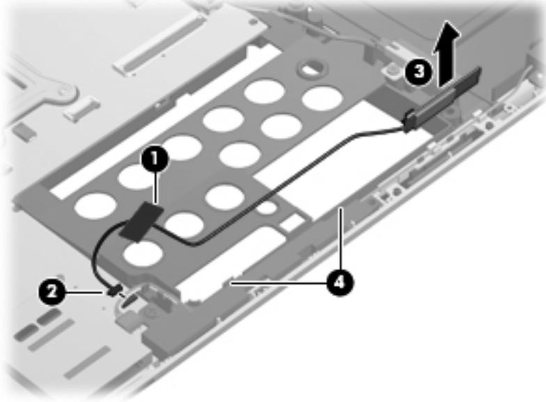
Reverse the above procedure to install the Bluetooth module.
