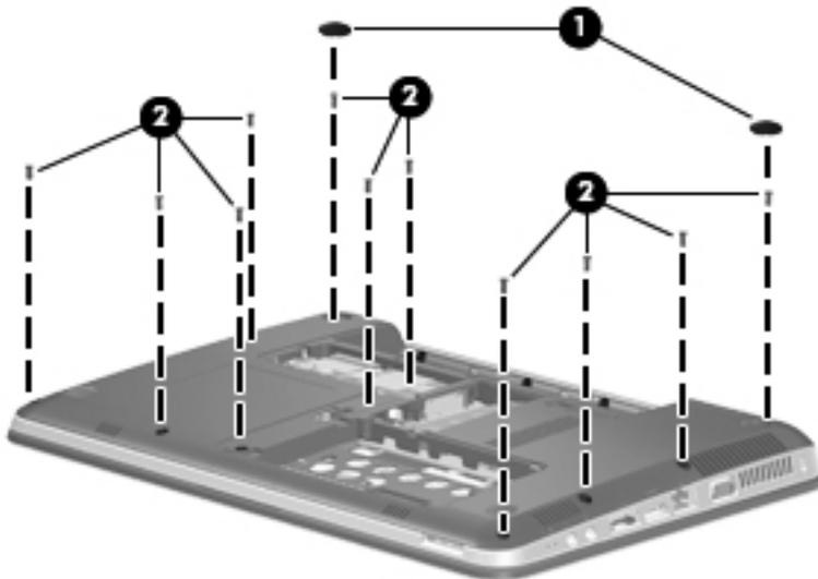
3. Remove the six Phillips PM2.0x2.0 broadhead screws that secure the top cover to the base enclosure.
