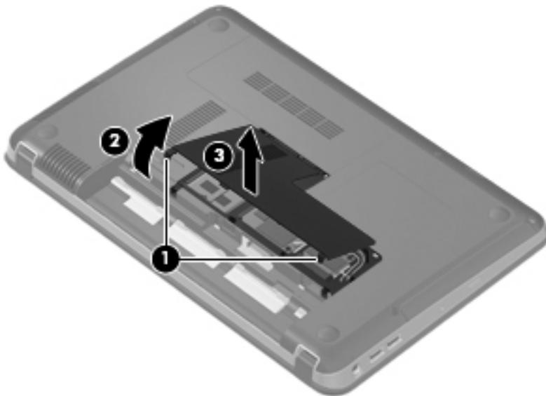
4. Spread the retaining tabs **(1)** on each side of the memory module slot to release the memory module. (The edge of the module opposite the slot rises away from the computer.)
