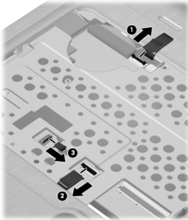
10. Remove the top cover from the base enclosure.
