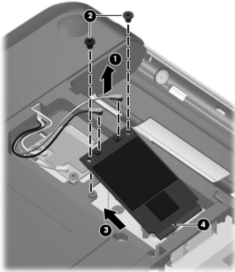
Reverse the above procedure to install the WWAN module.
