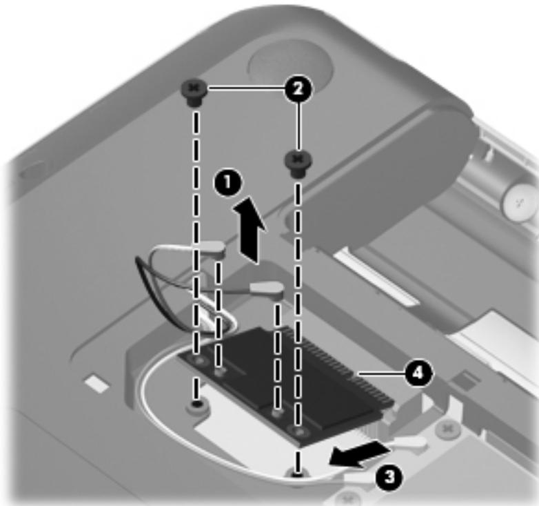
Reverse this procedure to install a WLAN module.
