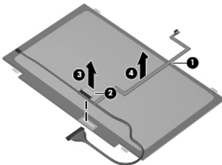
The display cable is available in the Display Cable Kit, spare part number 608211-001.
