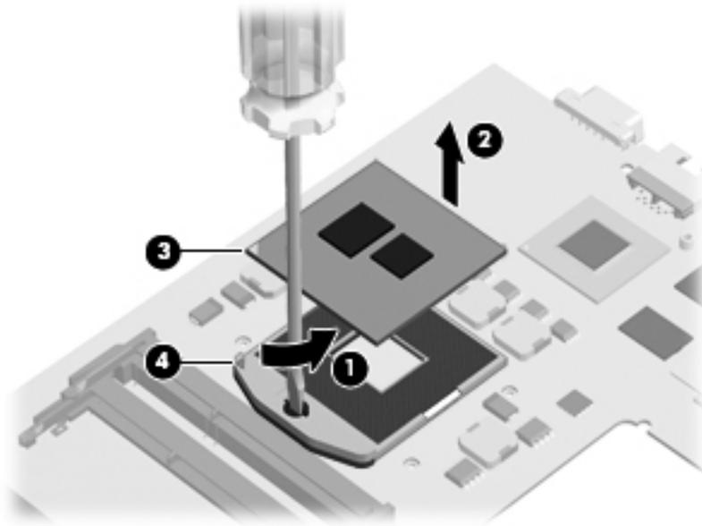
Reverse this procedure to install the processor.
