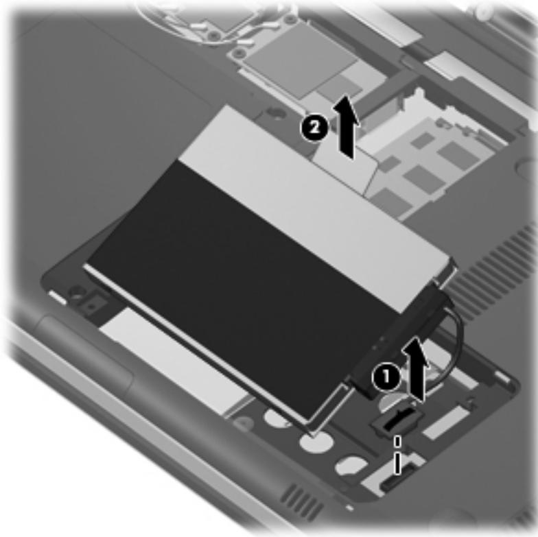
6. If it is necessary to replace the hard drive bracket (also called the protective cover), disconnect the hard drive cable (1) from the hard drive.
