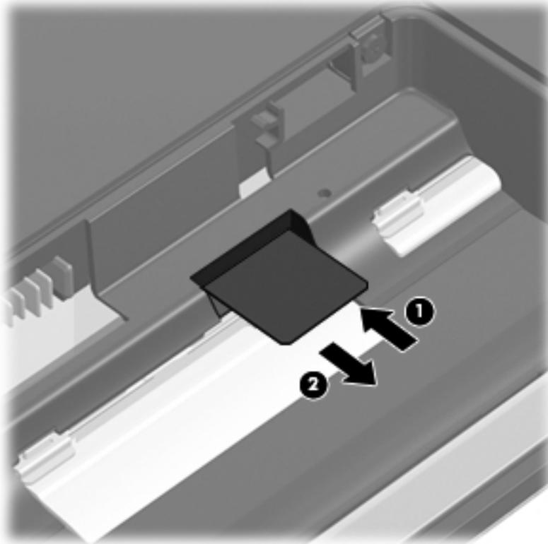
Reverse this procedure to install the SIM.
