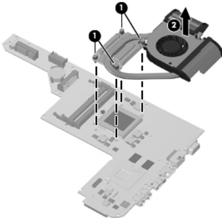
The thermal material must be thoroughly cleaned from the surface of the processor component (1) and the fan/heat sink assembly (2) each time the fan/heat sink assembly is removed. Thermal pads and thermal paste must be installed on all surfaces before the fan/heat sink assembly is reinstalled.
