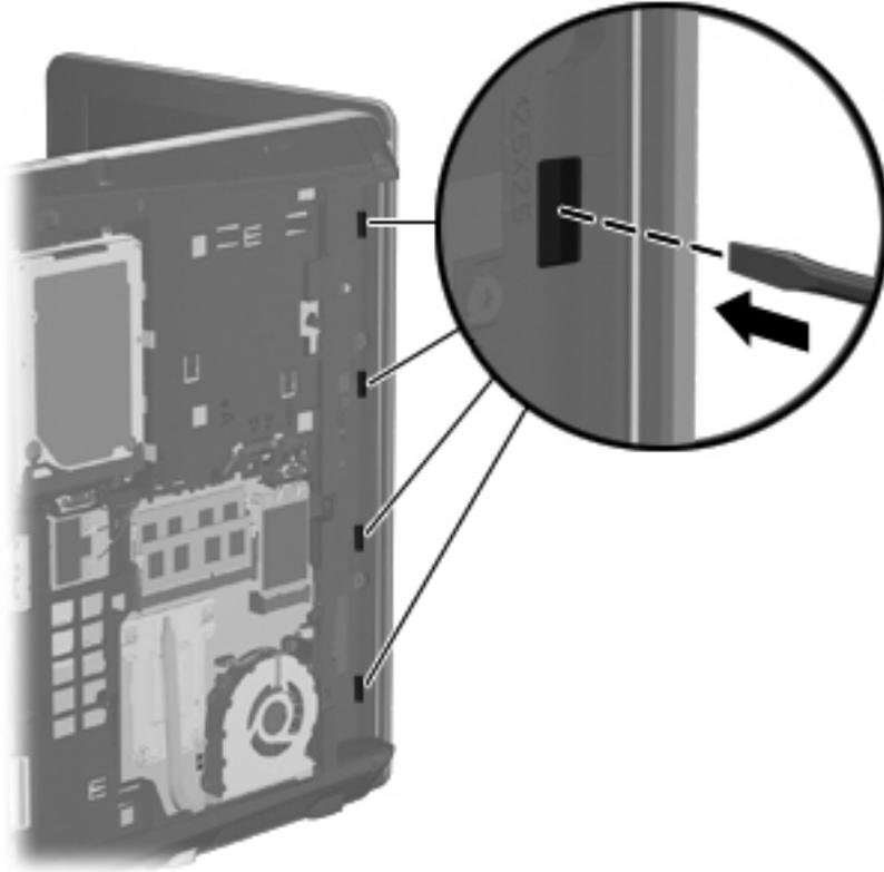
9. Pull up on the top of the top cover (1), pull upward on the left (2) and right sides (3), and then lift the top cover (4) enough to gain access to the audio board cable underneath.
