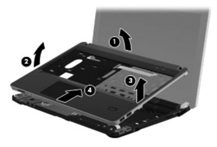
10. Under the top cover, open the system board connector (1), disconnect the audio board cable (2) from the system board, and then remove the top cover from the computer (3).
