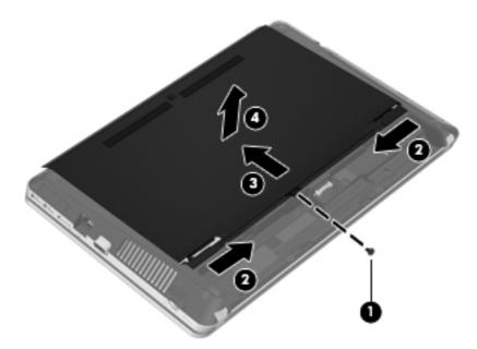
Reverse the removal procedures to install the bottom door.
