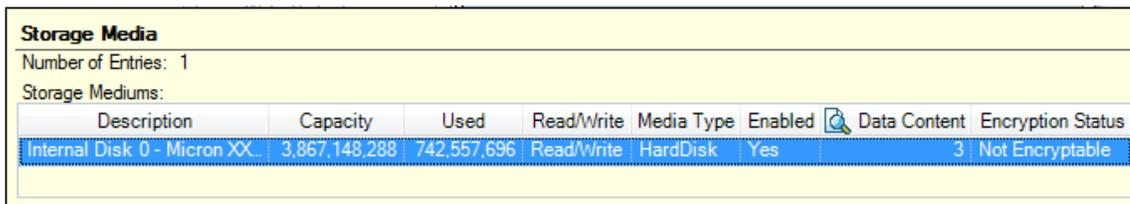
Figure 5: Shows the memory of a printer without a hard drive showing status of **Not Encryptable**
