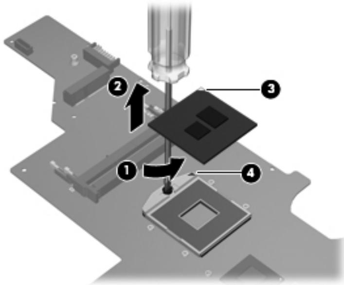
Reverse this procedure to install the processor.
