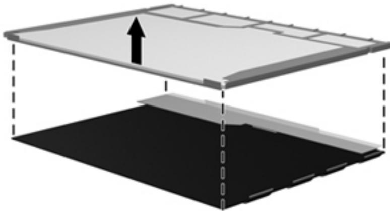
24. Recycle the LCD panel and backlight.
