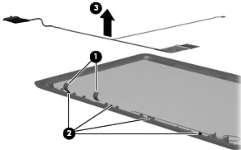
11. If it is necessary to replace the wireless antenna cable and transceiver:
