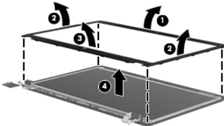
6. If it is necessary to replace the webcam/microphone module or microphone module:
