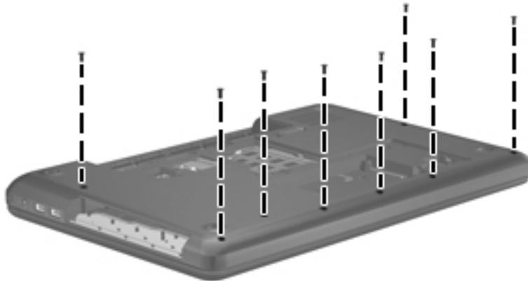
4. Remove the seven Phillips PM2.5×6.0 screws in the battery bay and the hard drive bay that secure the top cover to the computer.
