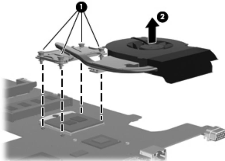
**NOTE:** The following illustration shows the fan/heat sink assembly removal process on a computer model equipped with an Intel processor, the Intel HM45 chipset, and a graphics subsystem with UMA memory.
