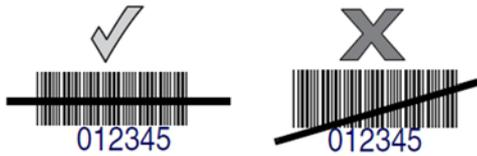
5. Do not hold the scanner directly over the barcode. Laser light reflecting directly back into the scanner from the barcode is known as specular reflection. This specular reflection can make decoding difficult. You can tilt the scanner up to  $65^\circ$  forward or back and achieve a successful decode.
