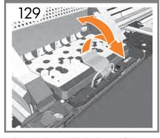
Pull up and release the blue latch on top of the carriage assembly to open the printhead cover.
