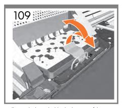
Pull up and release the blue latch on top of the carriage assembly. Lift the blue latch to open the printhead cover.
