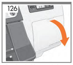
Pull open the printhead cleaning cartridge door, which is located on the right side of the printer.
