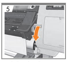
Lower the substrate-adjustment lever.
