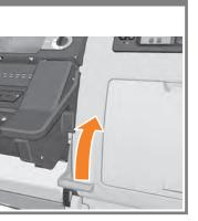
Insert the lead-edge of the substrate into the printer where shown.
