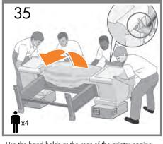
Use the hand holds at the rear of the printer engine to carefully lift the printer to its upright position so that the wheels with the anti-slip material touch the floor. HP recommends 4 people to complete this task.
