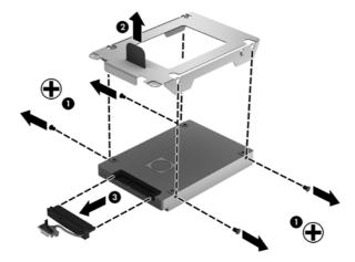
To install a hard drive, reverse this procedure.
