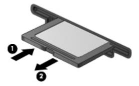
If the card is not ejected, pull the card out of the slot.
