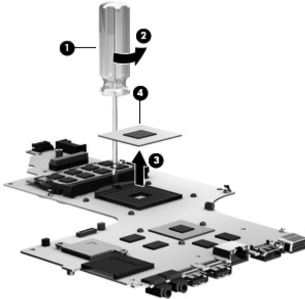
Reverse this procedure to install the processor.
