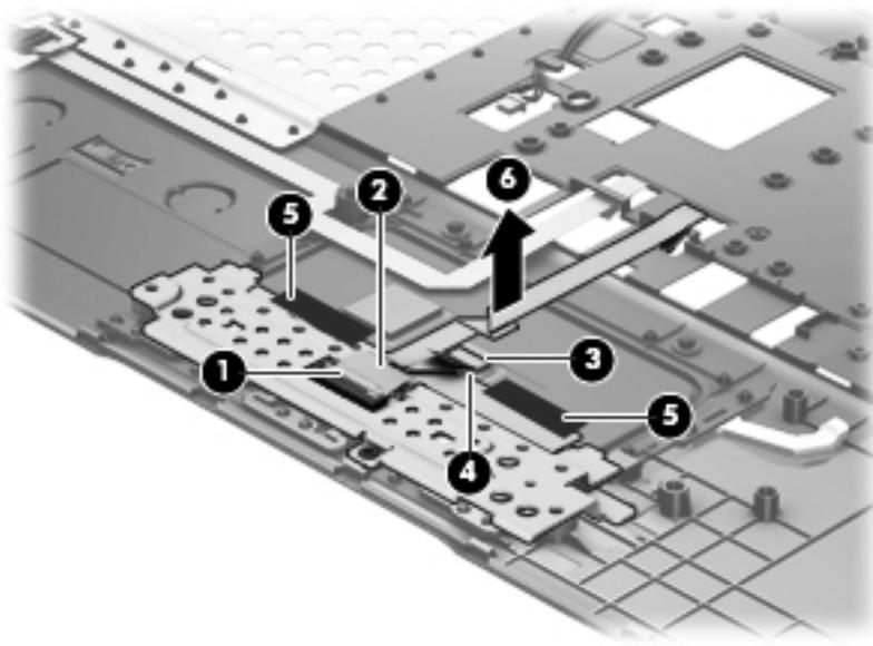
6. Remove the two Phillips PM2.5×4.0 screws **(1)** that secure the TouchPad button board bracket to the top cover.
