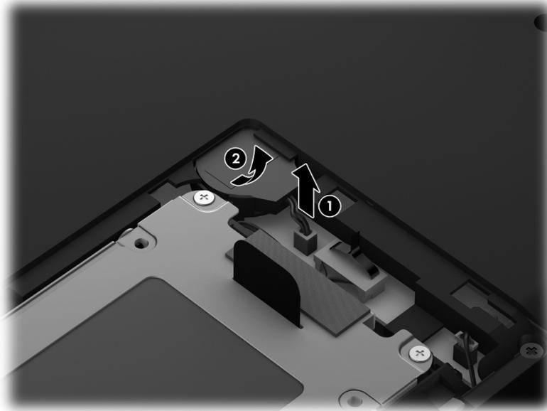
3. Remove the RTC battery.
