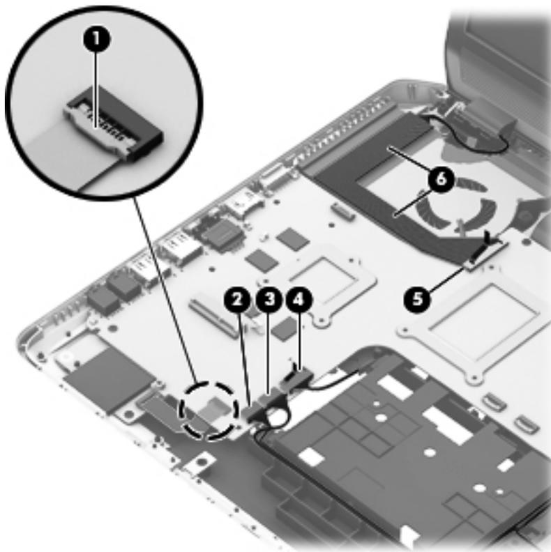
9. Disconnect the USB board cable (1) from the system board.
