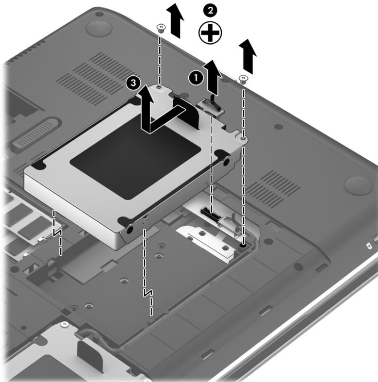
7. Disconnect the secondary hard drive connector cable **(1)** from the system board.
