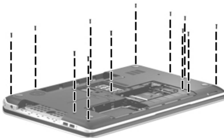
2. Remove the following screws that secure the top cover to the computer:
