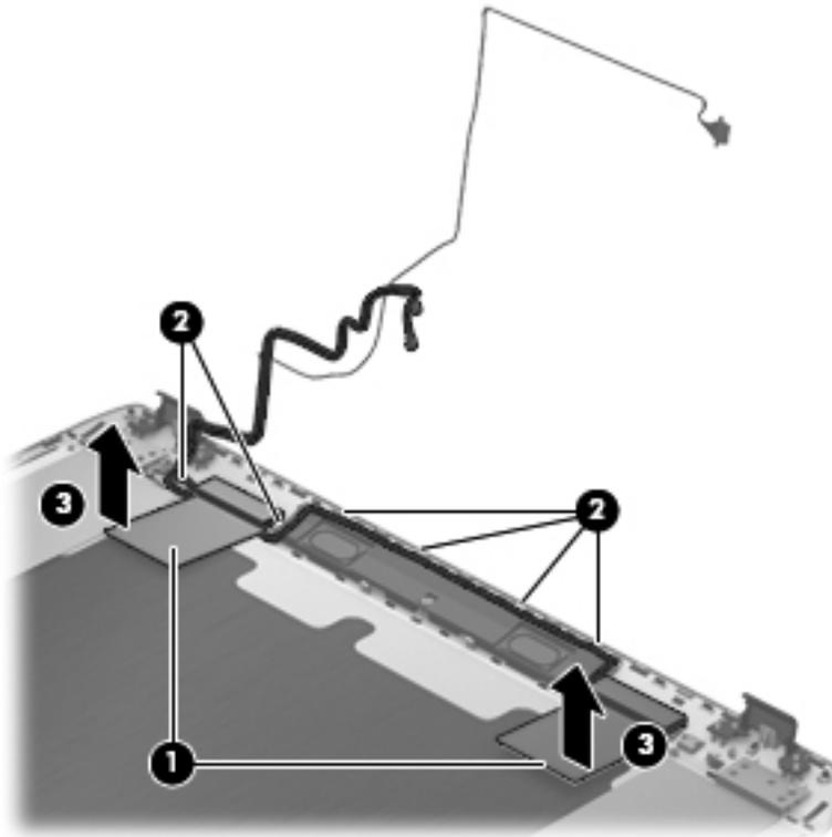
**13.** If it is necessary to replace the display speakers:
