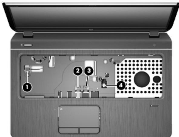
6. Remove the Phillips PM2.5×4.0 screw that secures the top cover to the computer.
