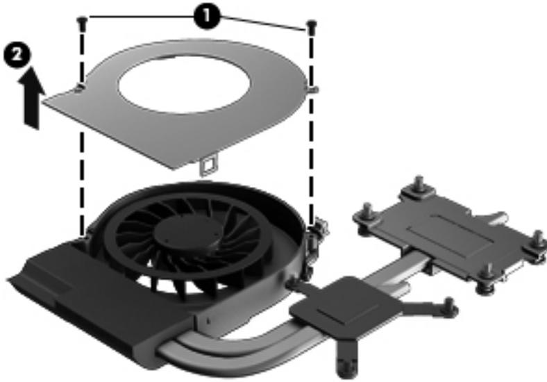
Reverse this procedure to reassemble and install the fan and heat sink.
