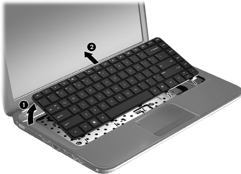
7. Tilt the keyboard forward (1) onto the palm rest. Release the zero insertion force (ZIF) connector (2) to which the keyboard cable is attached, and then disconnect the keyboard cable (3) from the system board.
