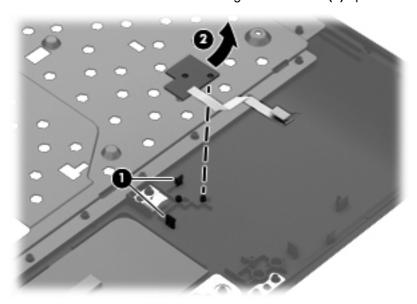
4. Remove the TouchPad LED board and cable.
