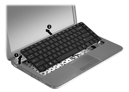
Tilt the keyboard forward (1) onto the palm rest. Release the zero insertion force (ZIF) connector **7**. (2) to which the keyboard cable is attached, and then disconnect the keyboard cable (3) from the system board.
