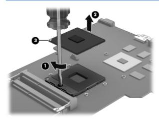
Reverse this procedure to install the processor.
