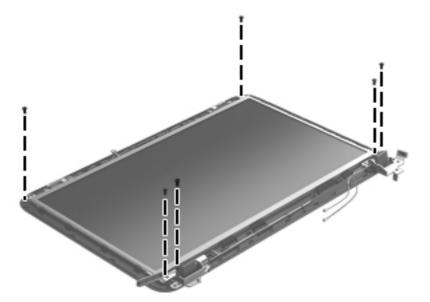
**b.** Lift the top edge of the display enclosure, **(1)** and then swing it up and forward until it is perpendicular to the display panel.
