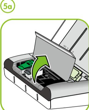
(EN) Install the ink cartridges. Once installed, the ink cartridges start initializing. They will stop moving when this process is complete.
