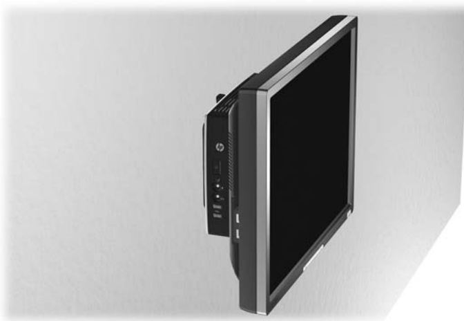
Figure C-5 Thin client mounted with flat panel on wall
