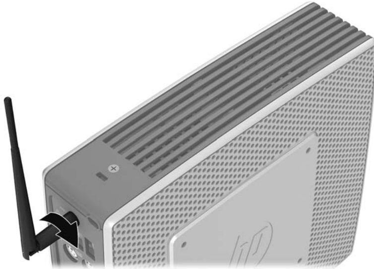
Figure 1-5 Installing the antenna
