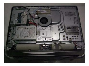
5. Remove the eight screws that attach the stand to the computer. There are four screws each at the bottom left and right of the computer. Save the screws.
