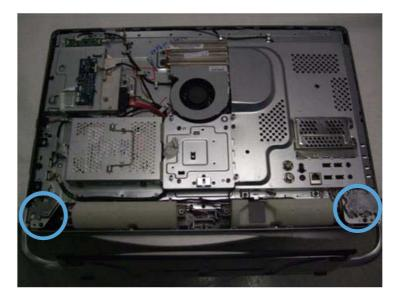
6. Install the four screws on both the left and right side to secure the stand to the computer.
