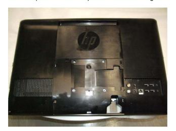
11. Attach the wall-mounting hardware (purchased separately) to the VESA adapter plate, according to the manufacturer's instructions, using the 100 mm x 100 mm screw holes.
