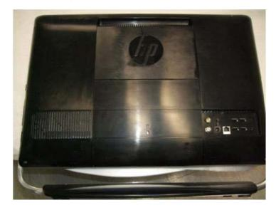
2. To remove the VESA cover, insert your finger into the slot and pry it off the computer.
