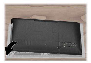
10. Tighten the two screws at the bottom of the computer to secure the back cover to the computer. If present, tighten the screw (1) at the center of the back cover.
