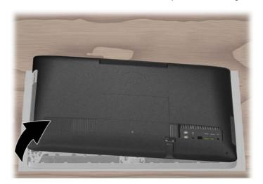
NOTE: You might have to exert force to remove the back cover from the computer. There might be a cracking sound as the back cover separates from the computer. The sound occurs when the latch hooks on the back cover slide off the latch bases on the computer.
