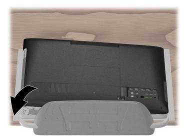
8. Tighten the two screws at the bottom of the computer to secure the back cover to the back of the computer. If present, tighten the screw (1) at the center of the back cover.
