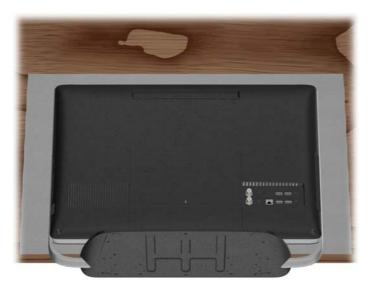
2. To remove the VESA cover, insert your finger into the slot just below the right bottom corner of the cover (1), and pry the cover off the computer (2). You might have to exert force to release the cover. Save the VESA cover.
