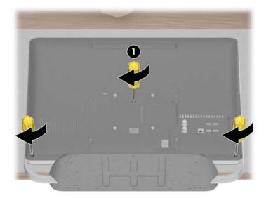
Replace the VESA cover on the back of the computer. Be sure to align the tabs on the VESA cover with the slots on the back of the computer and snap the cover into place.
