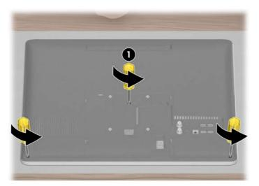
2. To remove the back cover from the computer, start lifting from the lower left corner.
