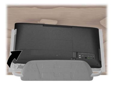
NOTE: You might have to exert force to remove the back cover from the computer. There might be a cracking sound as the back cover separates from the computer. The sound occurs when the latch hooks on the back cover slide off the latch bases on the computer.
