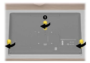
11. Attach the wall-mounting hardware (purchased separately) according to the manufacturer's instructions to the back of the computer, using the 100 mm x 100 mm (3.9 in. x 3.9 in.) screw holes.
