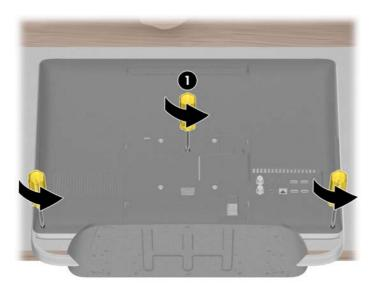
4. To remove the back cover from the computer, start lifting from the lower left corner.
