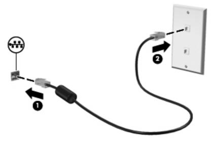
WARNING! To reduce the risk of electric shock, fire, or damage to the equipment, do not plug a modem cable or telephone cable into an RJ-45 (network) jack.
