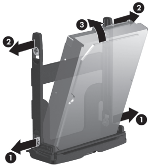
Figure 2 Attaching the hard drive to the drive carrier
