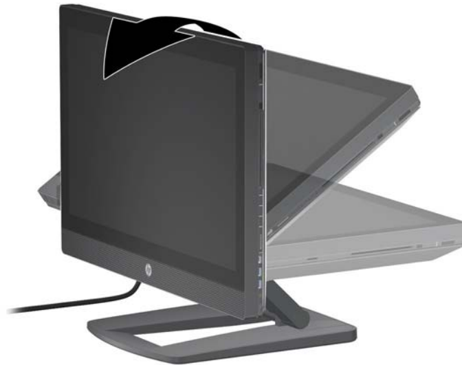
Figure 3-4 Redressement en position verticale
