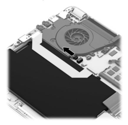
3. Move the battery cable to the side (1), and then remove the 3 Phillips PM 2.5×4.2 screws (2) that secure the battery to the top cover.
