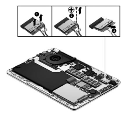
NOTE: If the WLAN antennas are not connected to the terminals on the WLAN module, the protective sleeves must be installed on the antenna connectors.
