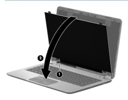
9. Release the support strip (1) that secures the display panel connector. Disconnect the display panel cable from the display panel (2), and then remove the panel (3).
