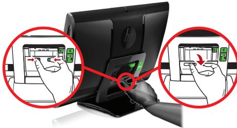
2. Reach into the rear cavity framed by the computer stand, and plug the power cord into the power connection at the top right corner.
