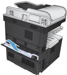
3. Place the attached cap over the opening on the front of the unit.
