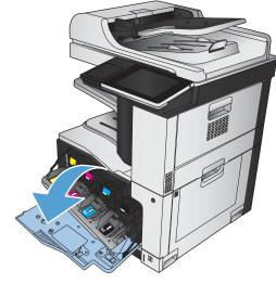
Grasp the handle of the used toner cartridge and pull out to remove.
