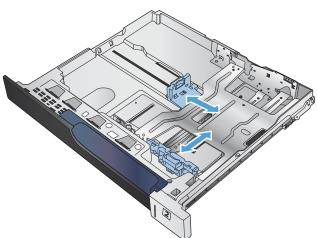
Load paper into the tray. Check the paper to verify the guides lightly touch the stack, but do not bend it.
