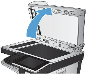
Clean the main scanner glass, the document-feeder glass (the small strip of glass on the left side of the scanner), and the white foam backing. Use a soft cloth or sponge that has been moistened with nonabrasive glass cleaner. Dry the glass and white plastic backing by using a chamois or a cellulose sponge to prevent spotting.
