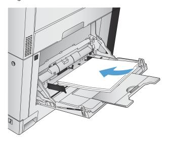
Make sure that the stack fits under the tabs on the guides and does not exceed the load-level indicators.
