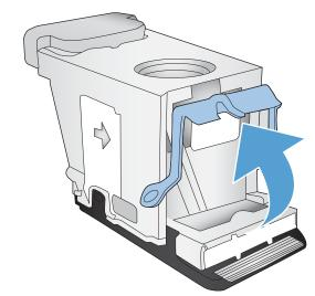
4. Remove the sheet of staples from the staple cartridge.
