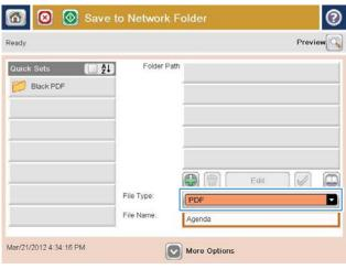
Touch the Add putton that is below the Folder Path field to open a keyboard, and then type the path to the network folder. Use this format for the path:
