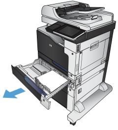
**ENWW** Clear jams 245 If the edge of the paper is visible in the feed area, slowly pull the paper down and out of the product.
