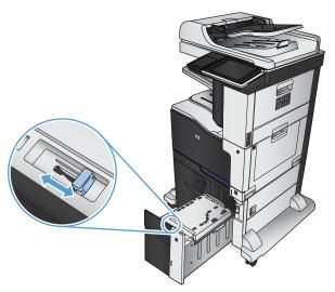
Load full reams of paper into each side of the tray. The right side holds 1,500 sheets of paper. The left side holds 2,000 sheets of paper.
