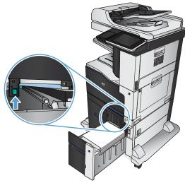
4. If jammed paper is in the feed area, pull it down to remove it.
