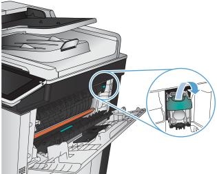
3. Insert the new staple cartridge into the opening. Press down on the top of the staple cartridge until it clicks into place.
