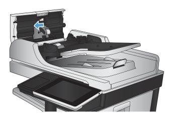
Lift the jam-access door, and remove any jammed paper.
