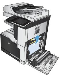
If paper is visible entering the bottom of the fuser, gently pull downward to remove it.
