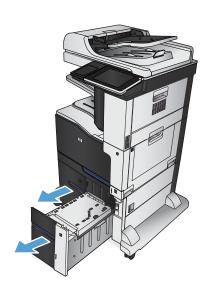
2. Remove any damaged sheets of paper.
