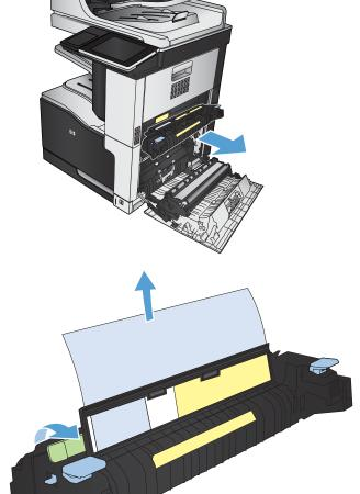
6. Align the fuser with the slots in the product, and push it straight in until it clicks into place.
