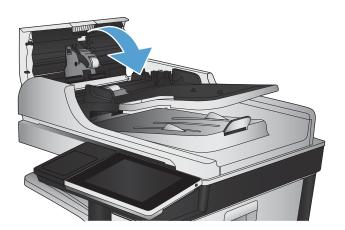
NOTE: To avoid jams, make sure the guides in the document feeder input tray are adjusted tightly against the document. Remove all staples and paper clips from original documents.
