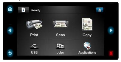
The front panel has a large central area to display dynamic information and icons. On the left and right sides you can see up to five fixed icons at different times. Normally they are not all displayed at the same time.
