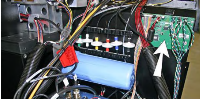
Figure 30 Vacuum reservoir or accumulator in H-series, visible at center. The board at the right is unrelated to the vacuum system.
