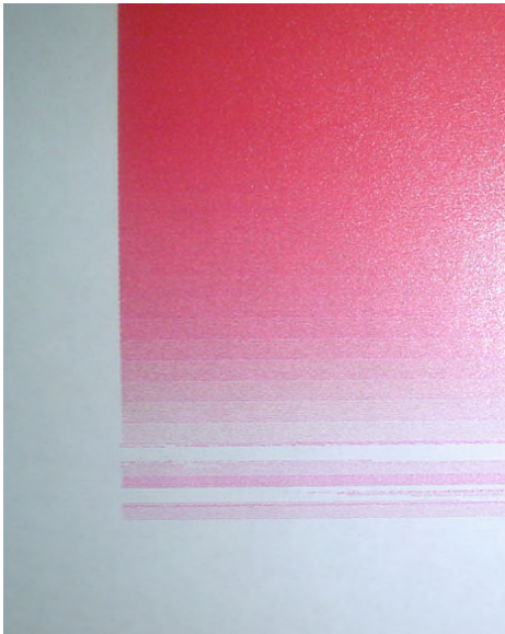
Figure 33 Detail of color coming back in following the drop out
