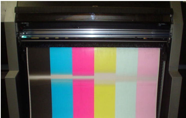
Figure 32 Output from H-series showing all colors fading away and then coming back
