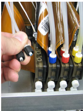
Figure 24 Both air tubes removed from a printhead in an H35100.
