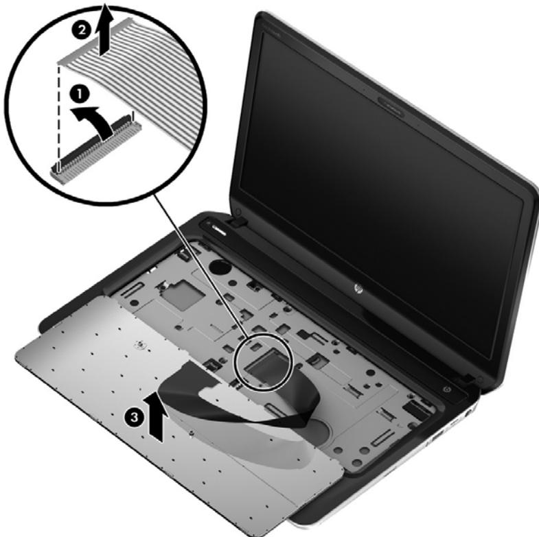
Reverse this procedure to install the keyboard.
