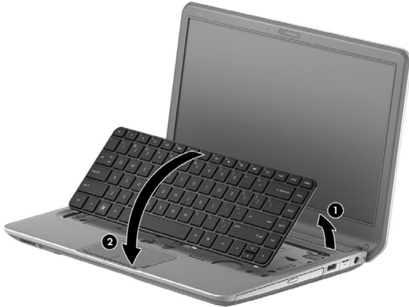
7. Release the ZIF connector (1) to which the keyboard cable is connected, and then disconnect the keyboard cable (2) from the system board.
