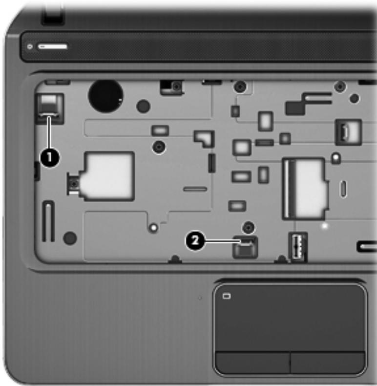
8. Remove the six Phillips M2.5×6.5 screws (1) that secure the top cover to the computer.
