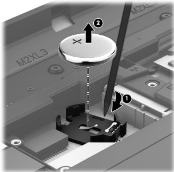
3. Remove the RTC battery.
