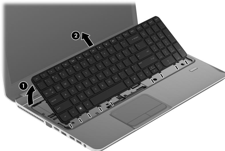
7. Lift the left side of the keyboard **(1)** until the keyboard cable and the keyboard backlight cable are accessible.
