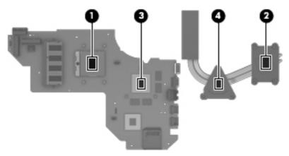
The following illustration shows the replacement thermal material locations on a computer model equipped with a graphics subsystem with discrete memory. Thermal paste is used on the processor (1) and the heat sink section (2) that services it.
