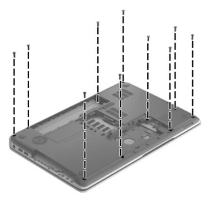
2. Remove the three Phillips PM2.0×2.0 broad head screws that secure the top cover to the computer.
