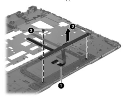
Reverse this procedure to install the TouchPad button board.
