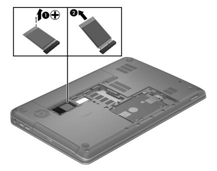
Reverse this procedure to install the solid-state drive.
