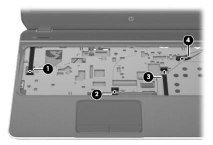
**6.** Remove the four Phillips PM2.5×5.0 screws that secure the top cover to the computer.
