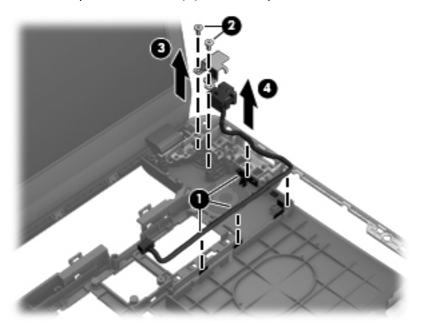
5. Remove the power connector cable.
