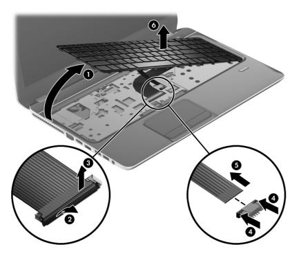
Reverse this procedure to install the keyboard.
