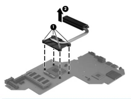
NOTE: The thermal material must be thoroughly cleaned from the surfaces of the heat sink and the system board components each time the heat sink is removed. Replacement thermal material is included with the heat sink, processor, and system board spare part kits.
