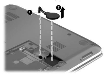
3. Remove the RTC battery.
