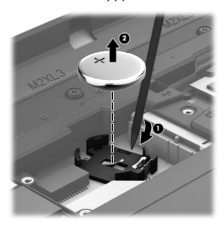
3. Remove the RTC battery.
