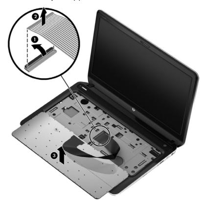
Reverse this procedure to install the keyboard.
