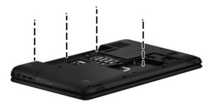
3. Remove the four Phillips PM2.5×4.0 screws on the front edge of the battery bay and near the hard drive connector that secure the top cover to the computer.
