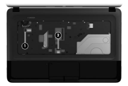
8. Remove the Phillips PM2.0×2.5 screw (1) and the three Phillips PM2.5×6.5 screws (2) that secure the top cover to the computer.
