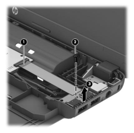
Reverse this procedure to install the USB board.
