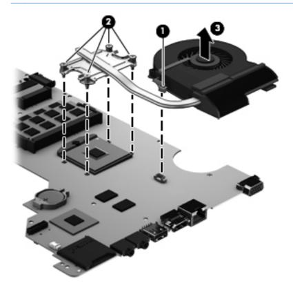
The thermal material must be thoroughly cleaned from the surfaces of the processor heat sink and the processor each time the processor heat sink is removed. Replacement thermal material is included with the processor heat sink and system board spare part kits.
