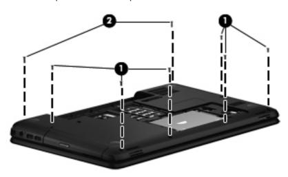
2. Remove the four Phillips PM2.0×2.5 screws on the rear edge of the battery bay and in the hard drive bay that secure the top cover to the computer.
