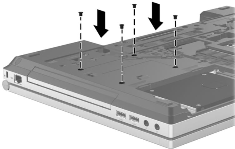
3. Replace the service door (see [Replacing the service door on page 34](#)).
