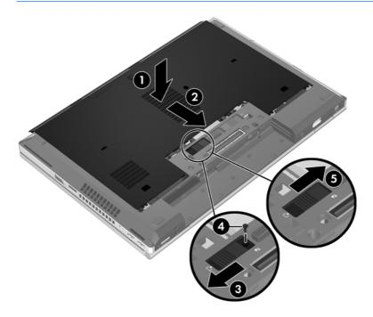
5. Insert the battery (see <u>Inserting or removing the battery on page 32</u>).
