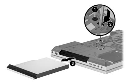
To install an optical drive in the upgrade bay:
