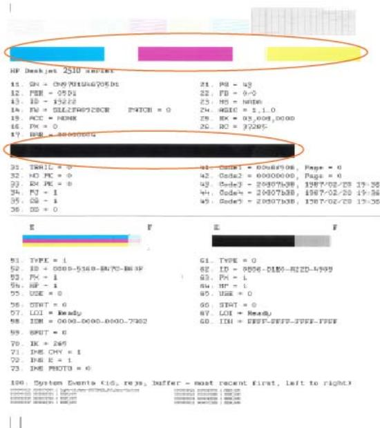
6. Clean the print cartridges automatically, if the diagnostic page shows steaks or missing portions of the color and black boxes.
