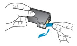
c. Slide cartridge into slot until it clicks into place.
