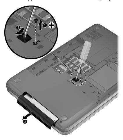
Remove the 2 PM  $2.0 \times 3.0$  screws (1) that secure the ODD bracket to the ODD and then remove the bracket (2) from the ODD.
