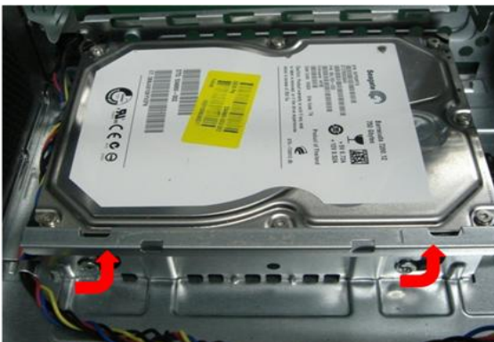
Figure 5-10 Hard drive screws
