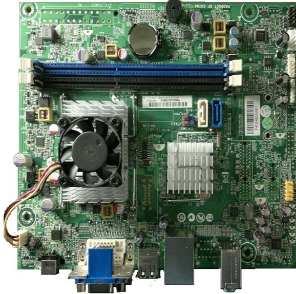
Figure 5-3 DIMM Socket Locations – 100B SFF PC
