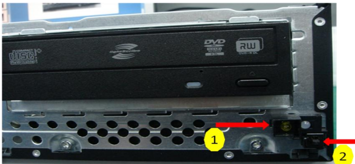
Figure 5-14 Removing the power switch
