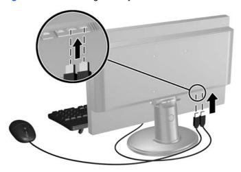
3. Connect a VGA cable between the VGA connector on the PC and the VGA connector on the rear of the monitor.
