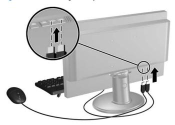
4. Connect one end of the power cord to the AC power connector on the back of the monitor and the other end to an electrical wall outlet.
