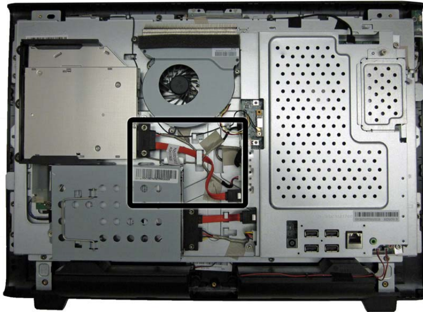
Figure 6-38 Optical drive cable location
