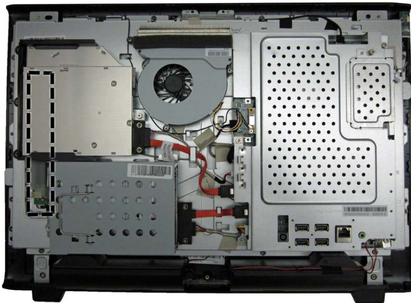
Figure 6-41 Inverter board location
