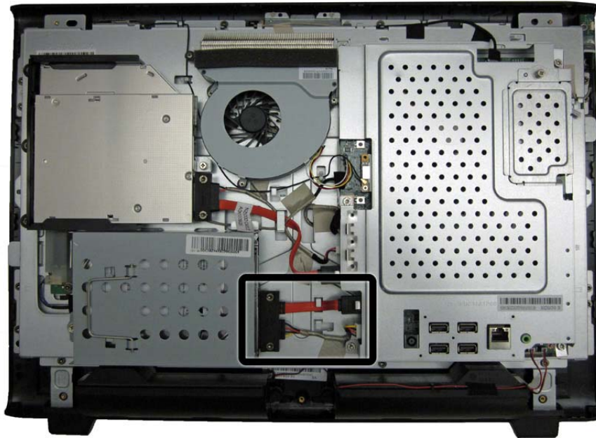
Figure 6-36 Hard drive cable location
