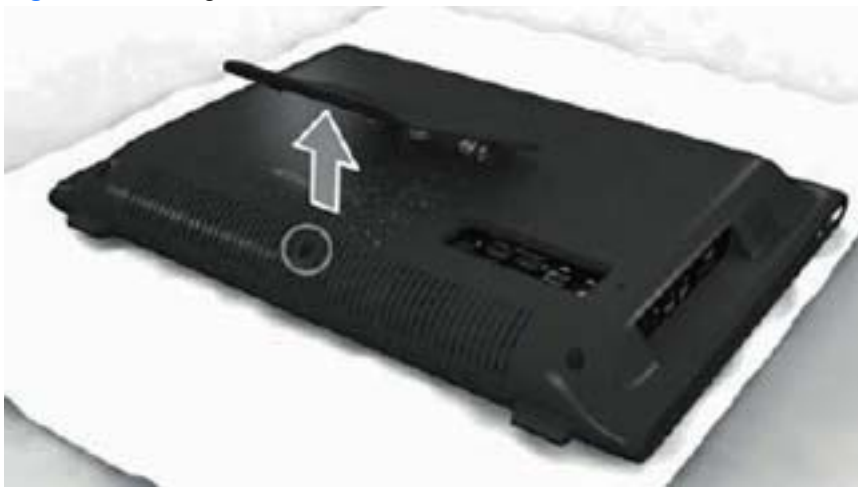
Figure 6-1 Lifting the stand
